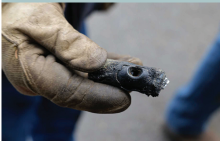
Section of underground line removed during repairs in Kala Point.
