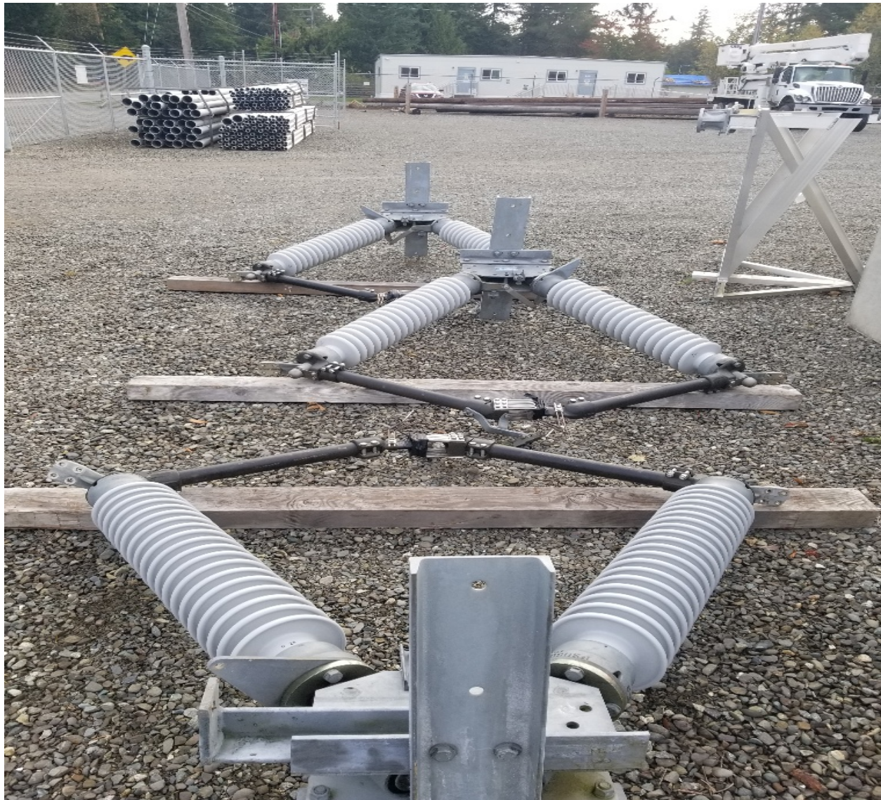
115kV switches old and burned up. Located at 210 Four Corners Road storage yard.
